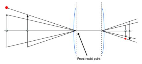
We believe that diagrams like this last one have contributed much to the confusion about the no-parallax point. There is no debate that these rays are correctly drawn, and faced with this diagram, it seems obvious that we must rotate around the front nodal point. What other point could we rotate around, that would keep the red dot and the black arrowhead lined up with each other?
