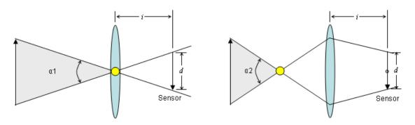
These two diagrams correspond to figures 2b and 2d shown earlier, but here we emphasize the angle of view subtended by the solid arrow, which fills the sensor. Notice that both diagrams show the same object, sensor, and lens, with everything in exactly the same place except for the aperture. And yet, on the left diagram the angle of view  $\alpha 1$  is about 37 degrees, while in the right diagram the angle of view  $\alpha 2$  has increased to about 68 degrees.
