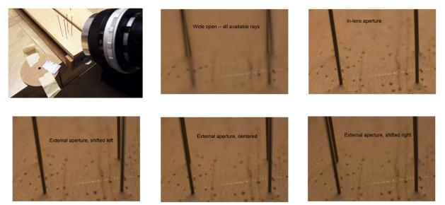
Figure 3. Experimental demonstration of shifting perspective by moving the aperture.
