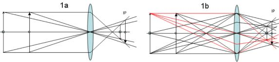
Figure 1. Ray Tracing a Thin Lens
